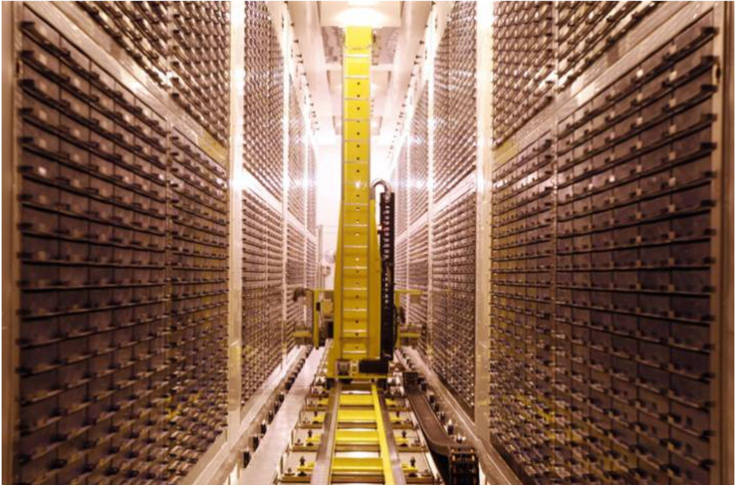
A storage robot deposits samples in a blood and urine sample freezer at Biobank, near Manchester, northern England.
